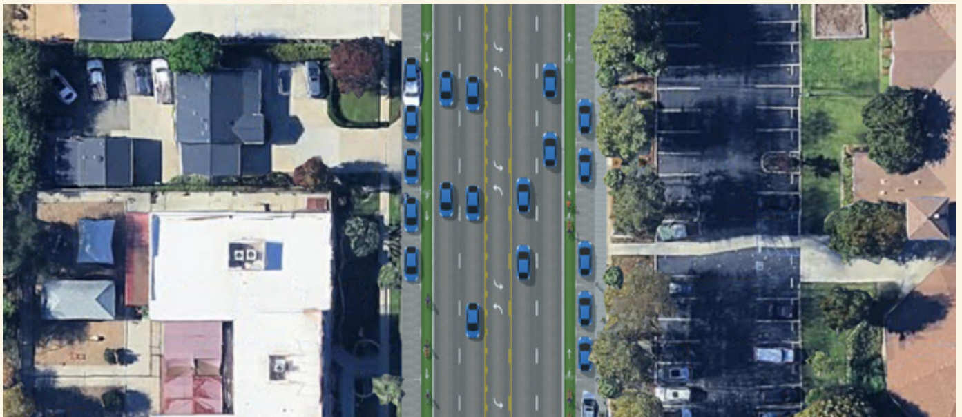
Exhibit 41. Proposed cross-section and overhead view for Bonita from Siglesia St to San Dimas Canyon Rd - looking east
