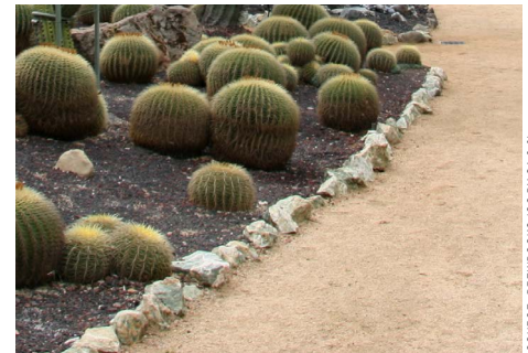
FIG. 11.E.3: AGGREGATE EDGE This aggregate path is retained at the edge by a row of cobbles
